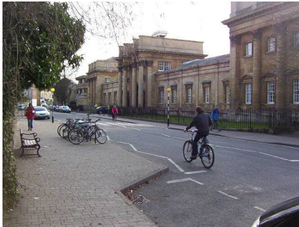
Cycle parking on Footway extension, Oxford
