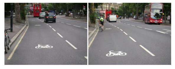
On this two lane stretch of road the inside lane was rarely used by motor vehicles. The cycling officer wanted to remove this lane and replace it with kerb build outs and a wide cycle lane but this was rejected by the traffic manager on 'capacity' grounds. Painting logos in the centre of the little used lane instead gives cyclists the confidence to assert themselves in this lane and sends a strong message to drivers that cyclists have a right
