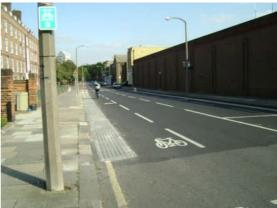
Instead of following the kerbline, the cycle lane takes a straight line based on the optimum Bikeability position. The remaining gap between the inside line of the cycle lane and the kerb is filled in with cobble effect imprint paving so that the cycle lane does not appear so wide that it would look like a general carriageway lane. The imprint also discourages cyclists from hugging the kerb whilst giving them space to do so in an emergency; this is a Bikeability concept.
