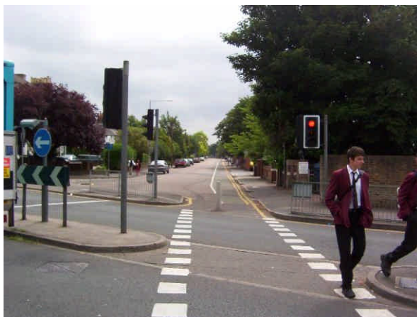
Signalised cycle crossing leading from town centre to quiet street High Street East, Slough
