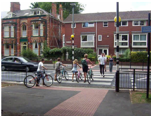
Pedestrians and cyclists share wide Zebra crossing. Note 'Cyclists dismount' sign top right of picture, Hull
