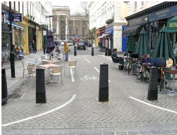
Road closure and redistribution of carriageway achieved by bollards – London
