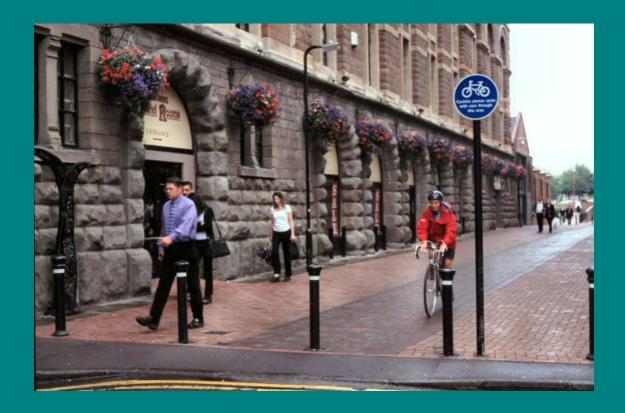
Back to the UK. The non-standard sign reads 'Cyclists please cycle with care through this area'. While not completely 'invisible', the provision for cyclists here is relatively subtle. Note the lack of Give-Way markings where the cycle route rejoins the carriageway, acknowledging that the vast majority of riders do possess a modicum of common sense and self-preservation.
