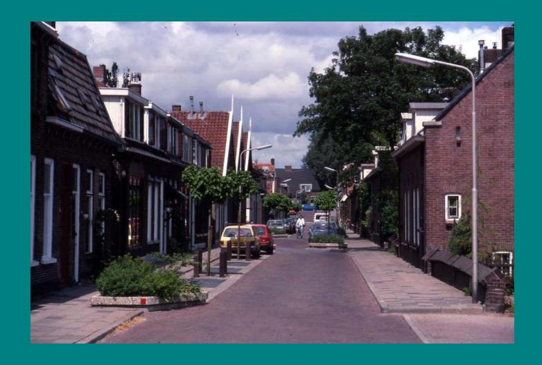
A home zone style treatment, this illustration from the Netherlands. The limited road width, interrupted forward visibility and soft landscaping create an obvious impression that low vehicle speeds are appropriate, creating an attractive environment for walking and cycling. Note the almost complete absence of signing and lining.
