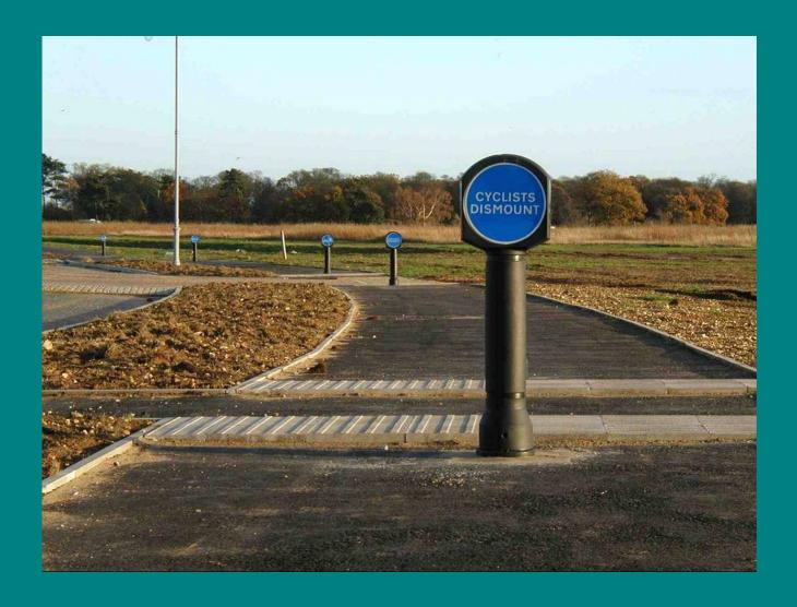
Another example of where poorly designed cycle 'facilities' have generated visual clutter, here within the highway layout of a new residential development. Not to mention the unhelpfulness of all those closely spaced Cyclists Dismount signs! Why not keep cyclist on the adjacent quiet access road where they would maintain priority across side turnings and obviate the need for the succession of (likely to be ignored) 'Cyclists Dismount' bollards
