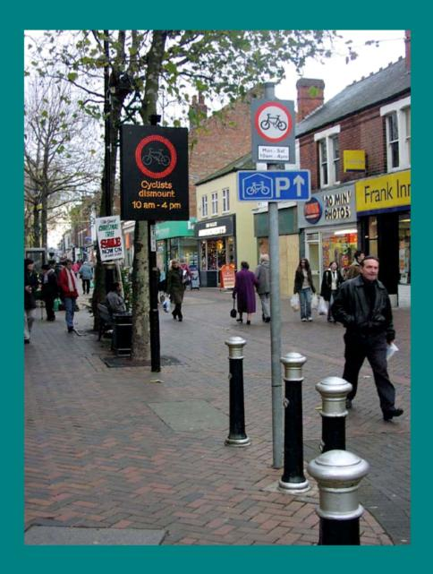
The variable message sign lights up each time a cyclist approaches it during the core shopping period when cycling is prohibited. Is the treatment reaction proportionate to the seriousness of the 'offence'? What would a better design solution have been?
