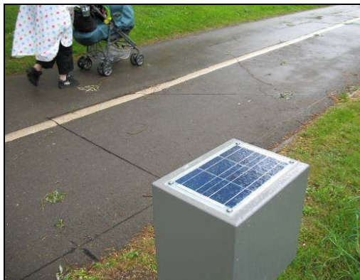
Counter cabinets and solar panels at loop detector sites
