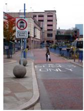
Something of a potential mixed message here. While the surface markings indicate that both buses and cycles are permitted to enter this street, the adjacent signage makes no 'overt' mention of a way through for people using bikes. The no motor vehicle ('flying motorbike') sign is often misinterpreted as applying to all traffic, including cycles.
