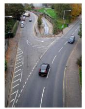
An example of a junction layout that is not at all cycle-friendly, here at the junction of Hamilton Street and Albert Street. The wide junction mouth and sweeping bend enable (particularly left turning) motorists to negotiate it at speed, endangering 'straighton' cycle movement. The junction geometry needs to be significantly tightened up.
