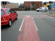
An advanced Stop Line at the junction of Montague Street with Whalley Banks. The central filter lane enables right-turning cyclists to access and gain a good position within the ASL, avoiding conflict with left turning vehicles. The red surfacing appears to discourage motorists from encroaching within cyclists' space, but is prone to erosion, and will need to be maintained if it is continue to remain effective.
