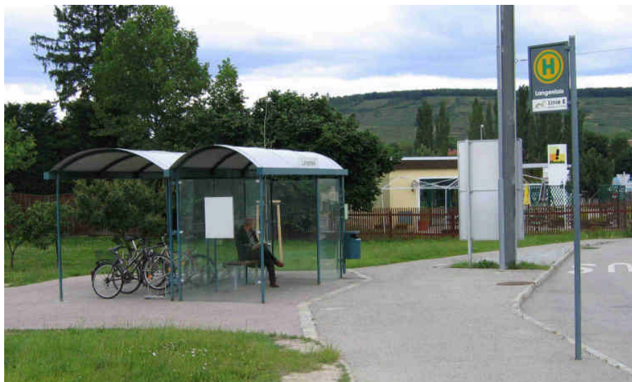
Cycle parking incorporated into the shelter at a rural bus stop in Langenlois, Austria
